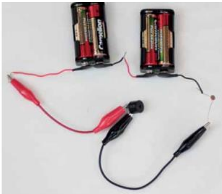
Figure 4: A circuit where the current is regulated by a light-dependent resistor
