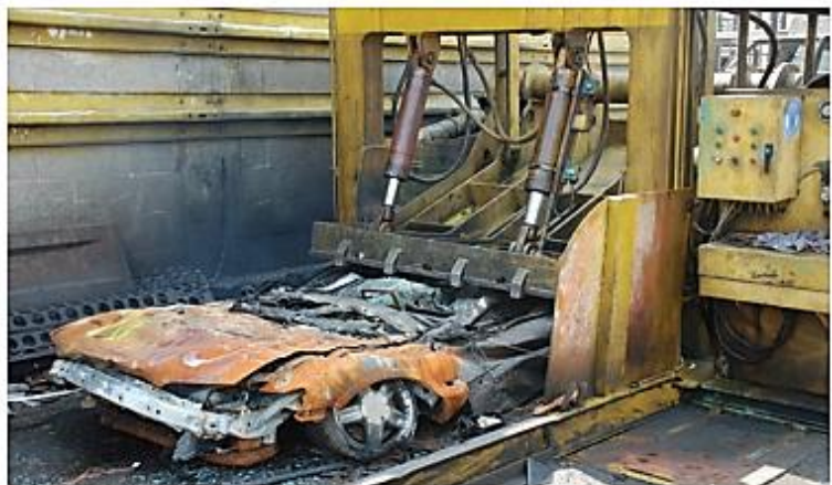
Figure 4.3 A hvdraulic car press crushes a car.
