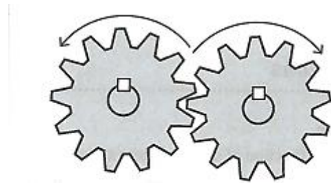
FIGURE 20 Spur gears of equal size, counter-rotating
