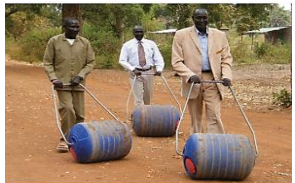
Figure 7 The Hippo Water Roller, designed by Petzer and Jonker, has improved the lives of many South Africans by making it easier to transport water.
