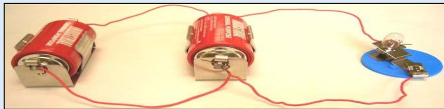
Parallel Circuit (Batteries in parallel)
