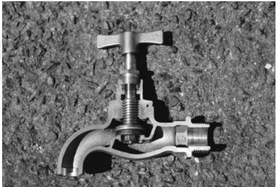
Figure 5.3.2: A cross section through a tap
